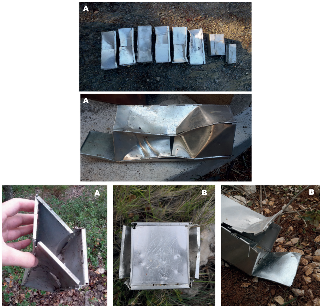
Fig. 1. A, small mammal traps damaged by wild boar in Collserola Natural Park. Sherman traps were more prone to serious damage than Longworth traps. The marks of the two lower incisors can be seen in the dented Sherman traps. B, damage caused by foxes V. vulpes (and other mesocarnivores) can be differentiated by the marking of the canines and by the bending of the extremes of the traps to gain access to the interior (Garraf Park).
