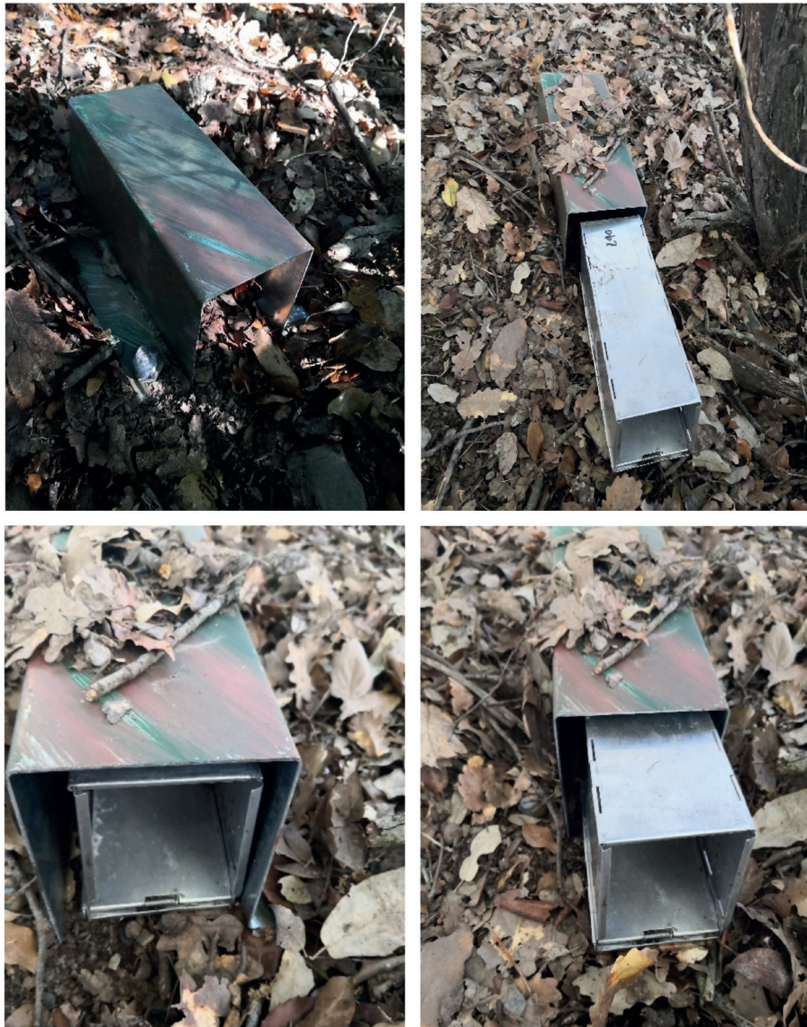
Fig. 4. Prototype protective guards against wild boar attacks made from galvanized steel. Their size allows insertion of small to medium-sized commercial traps (Longworth/Heslinga and medium-sized Sherman traps, the last shown in the photos).
