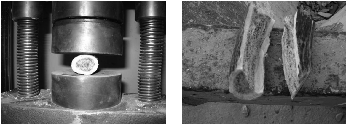
Fig. 2. Experimental setup for indirect tensile strength test (left). Result of its application to a cylindrical fragment from the antler of one of the deer (right).
